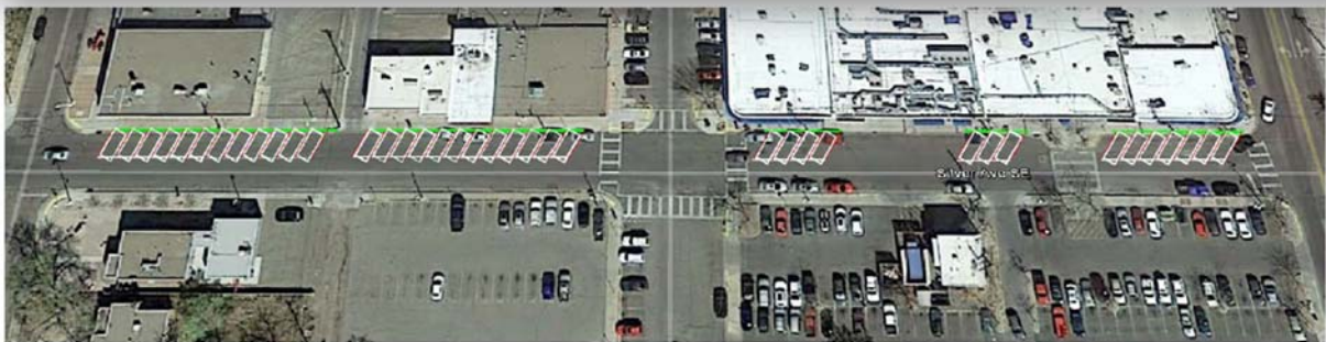
Parking on Silver in Nob Hill with 60 degree head-out angle parking - 38 legal spaces
