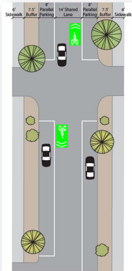
Figure 16 Proposed Cross Section from Girard to Tulane
