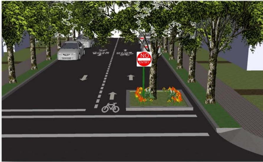
Figure 27 Preferred Layout for Diverter on Silver at Morningside
